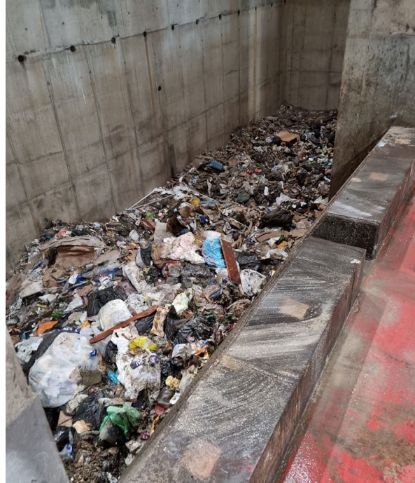
Waste in the reception bunker, where the waste is delivered to site via the council Bin wagons
